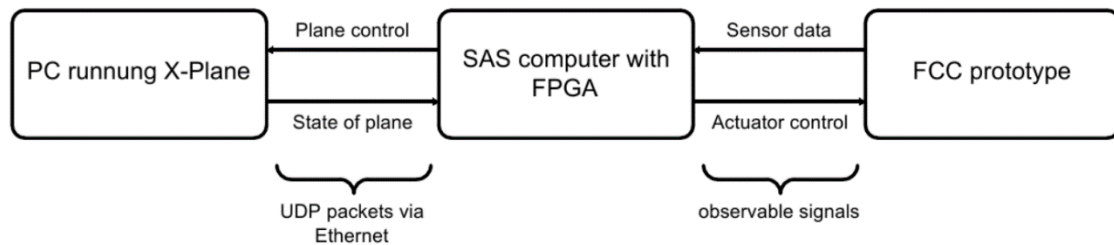
Figure 1. Basic concept of the HIL system
