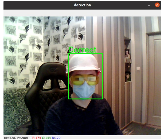
Fig. 5. The result in the presence of a white helmet, a blue medical mask and yellow goggles on the employee
