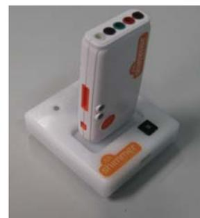
Figure 1: Shimmer3 device with charging station.
