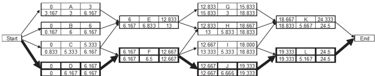
Fig. 3. The critical path due to PERT
