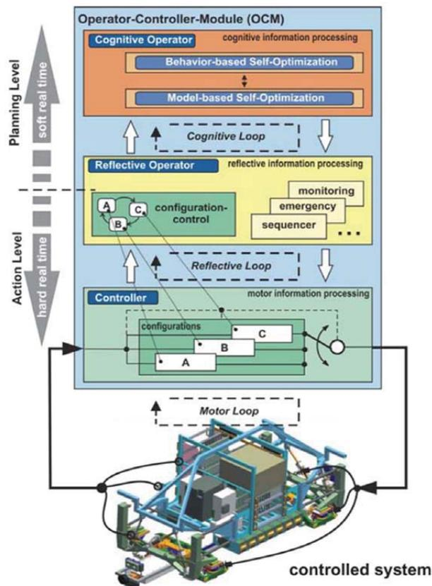
Fig. 6: Technology stack of the Operator-Controller-Module (OCM) [6,7]
