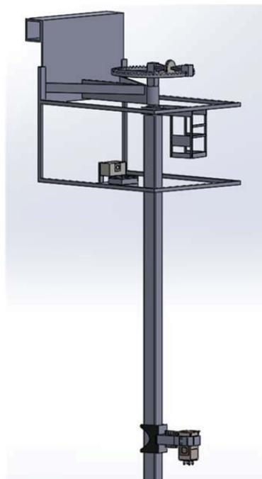
Fig. 4: Mast installation for sensor head within the biogas fermenter (test installation at university building)
